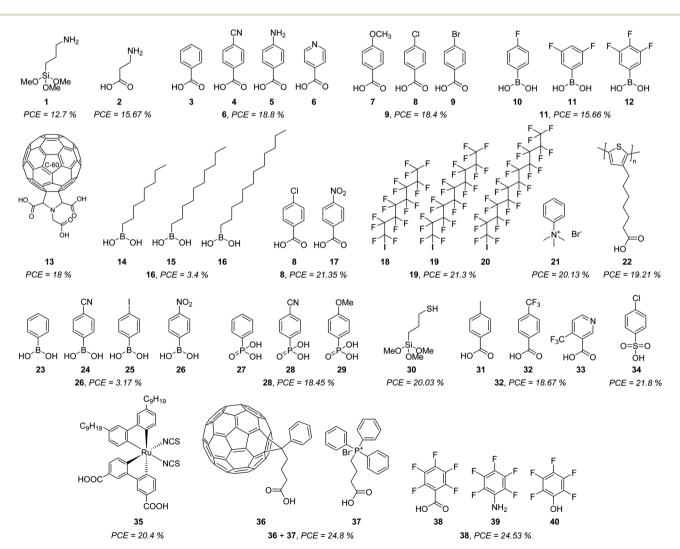
Fig. 4 Commercial molecules are used for the formation of SAMs in PSCs, indicating the highest PCE obtained in each case.
