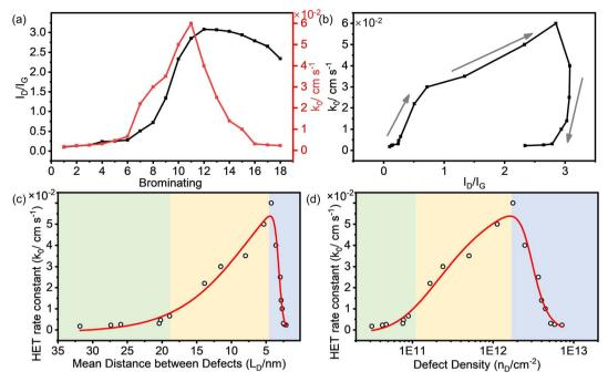
Fig. 3 (a) The  $I_D/I_C$  (black line) and the standard HET rate constant  $k^0$  (red line) varying with the continuation of the bromination process. (b) The correlation between  $I_D/I_G$  and  $k^0$ . (c and d)  $k^0$  as a function of defect density  $n_D$  (cm<sup>-2</sup>) and the mean distance between defects  $L_D$  (nm), respectively.
