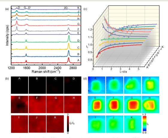
Fig. 2 (a) Raman spectra (vertically aligned) and (b) Raman  $I_D/I_G$  mapping of the brominated SLG patterns. (c) The probe approaching curves and (d) SECM images obtained on the brominated SLG patterns. In the SECM experiments, the tip electrode was held at a potential of 0.4 V in the electrolyte solution containing 1 mM FcMeOH and 0.1 M KCl, while the SLG substrate was kept unbiased. The tip-substrate distance was kept constant at 2.2  $\mu$ m (d/a = 0.44).
