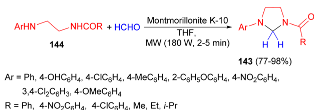
Scheme 47 Synthesis of 1-acyl-3-arylimidazolidines 143 using montmorillonite clay K-10.
