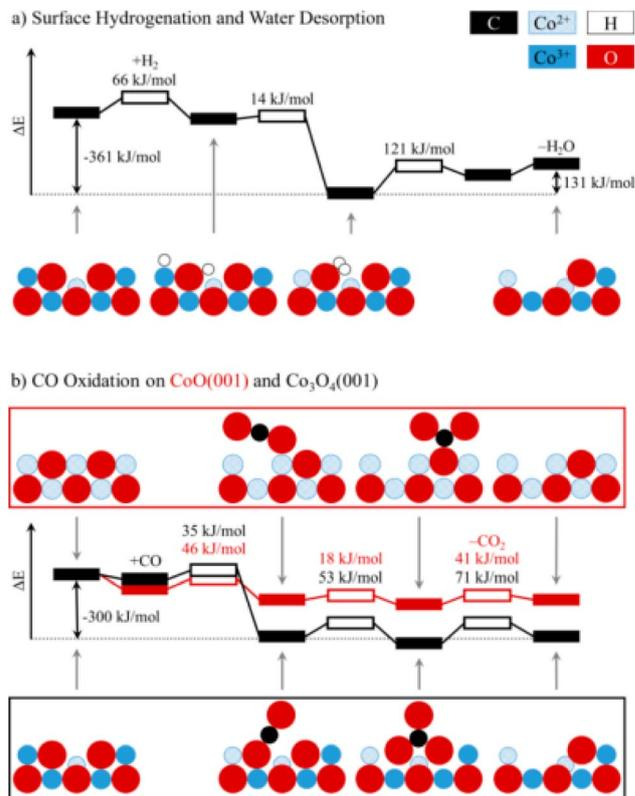
Fig. 12 Potential energy diagrams for (a) the hydrogenation of Co<sub>3</sub>O<sub>4</sub> {001} and (b) the oxidation of CO to CO<sub>2</sub> on Co<sub>3</sub>O<sub>4</sub> {001} and CoO {001}. For each transition state (hollow boxes), reaction barriers are given in kJ mol<sup>-1</sup>. Selected intermediates are shown as a side view along [110], using the following color codes: black (C), blue (Co), red (O), and white (H). Reprinted with Permission from ref. 90, 2019 American Chemical Society.
