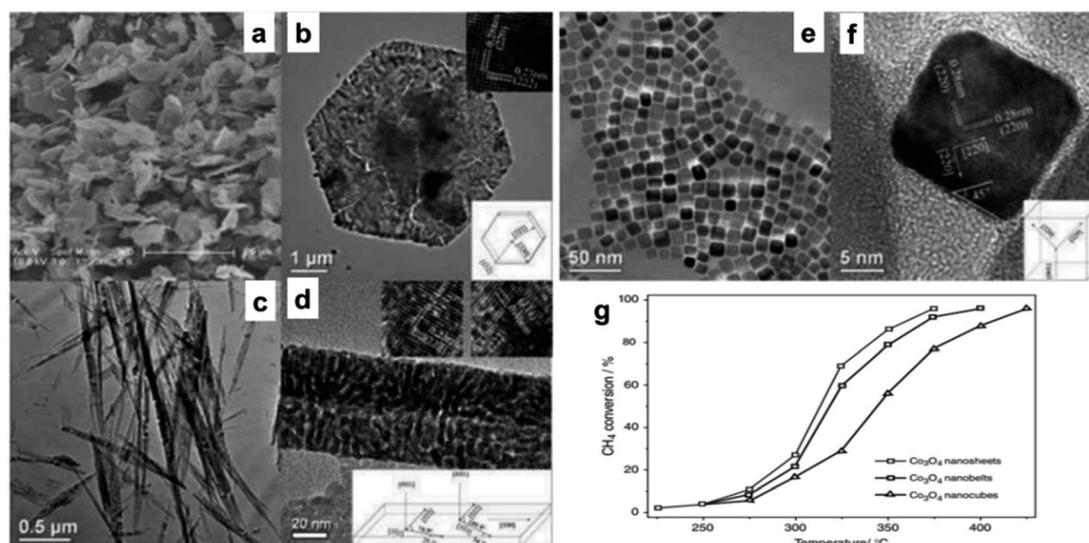
Fig. 2 Scanning electron microscopy (SEM) and high-resolution transmission electron microscope (HRTEM) analysis with structural models of  $\text{Co}_3\text{O}_4$  nanostructures: (a and b)  $\text{Co}_3\text{O}_4$ NS; (c and d)  $\text{Co}_3\text{O}_4$ NB; (e and f)  $\text{Co}_3\text{O}_4$ NC. (g) Methane conversion efficiency vs. temperature for  $\text{Co}_3\text{O}_4$  at a GHSV of  $40\,000 \text{ h}^{-1}$  (based on ref. 30, Copyright 2008, American Chemical Society).
