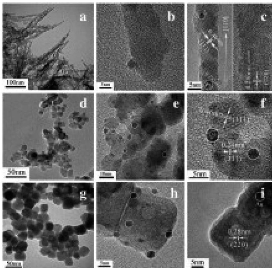
Fig. 8 Transmission electron microscope (TEM) images of  $\text{Co}_3\text{O}_4$ NR (a),  $\text{Co}_3\text{O}_4$ NH (d), and  $\text{Co}_3\text{O}_4$ NC (g). High-resolution transmission electron microscope (HRTEM) images of  $\text{Au}/\text{Co}_3\text{O}_4$ NR (b, and c),  $\text{Au}/\text{Co}_3\text{O}_4$ NH (e, and f), and  $\text{Au}/\text{Co}_3\text{O}_4$ NC (h, and i). Source: reprinted with permission from ref. 78, ©2011 Elsevier BV.
