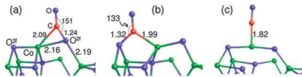
Fig. 11 Three adsorption configurations of CO on Co<sub>3</sub>O<sub>4</sub>(110): (a) on O<sup>2f</sup>; (b) on O<sup>3f</sup>; (c) on Co. Bond lengths are in angstroms; bond angle are in degrees. Co, green, O, blue, and C, red. Reprinted with Permission from ref. 88, 2011 Royal Society of Chemistry.
