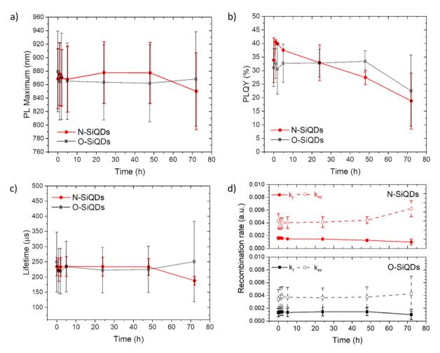
Fig. 3 A summary of the optical properties of N-SiQDs (red circles) and O-SiQDs (black squares). (a) PL maxima, (b) PLQY, (c) PL lifetime, and (d) recombination rate ratio as a function of time over a period of 72 h of UV irradiation. Error bars represent the 95% limit of measurement. Representative PL and UV-vis absorption spectra of each sample are plotted in Fig. S3, S4 and summarized in Tables S2, S3.†
