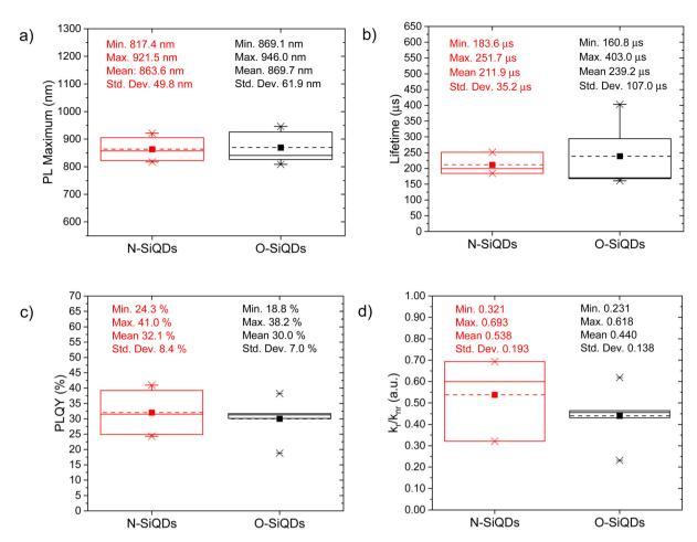
Fig. 2 Boxplots comparing the (a) PL max, (b) mean PL lifetime, (c) PLQY, and (d) k<sub>r</sub>/k<sub>nr</sub> of the as-produced N-SiQDs an5555d O-SiQDs. Mean and median of the distributions are represented by dash and solid lines in the boxes, respectively.
