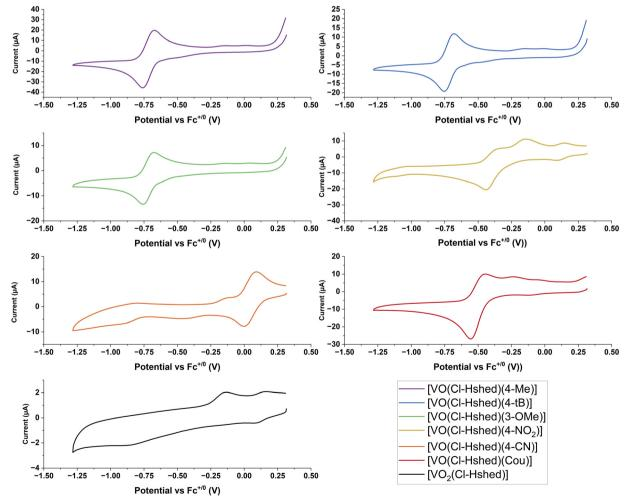
Fig. 7 Cyclic voltammograms of tested compounds at 2 mM in CH<sub>3</sub>CN in the presence of 0.1 M TBAP as the supporting electrolyte. Scans were cycled at 100 mV s<sup>-1</sup> from approx. 0.5 V vs. Fc<sup>+/0</sup> to -1.1 V using a glassy carbon working electrode.
