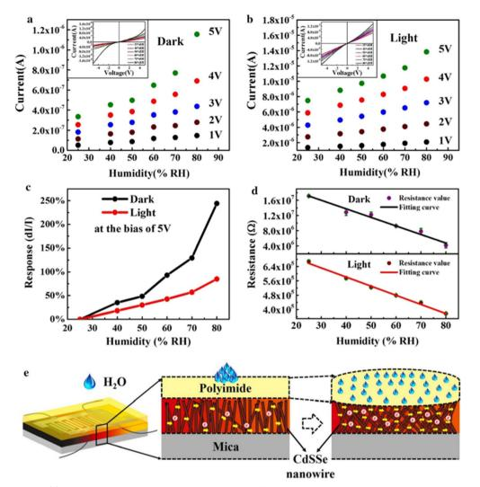
Fig. 14 (a) Dark current and (b) photo-current at various humidity levels under different bias and the inset shows the IV characteristics in the dark (a) and light (b) at different relative humidity. (c) Relative humidity-dependent moisture responsivity of the sensor in dark and bright fields, respectively. (d) Resistance at various relative humidity of the sensor in dark and bright fields, respectively. (e) Schematic theoretical diagram of humidity sensing by the sensor.188
