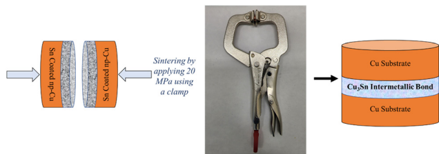
Fig. 1 Demonstrating the pressure application process, administered at high-temperature, using C-clamp locking pliers.
