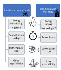
**Fig. 6** Comparison of the main aspects involved in traditional "dry" (solid-state reaction and milling) and "wet" (co-precipitation, sol–gel, solvothermal and electrodeposition) synthesis protocols.
