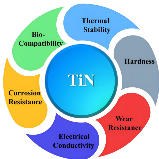
Fig. 2 Various properties of titanium nitride (TiN).
