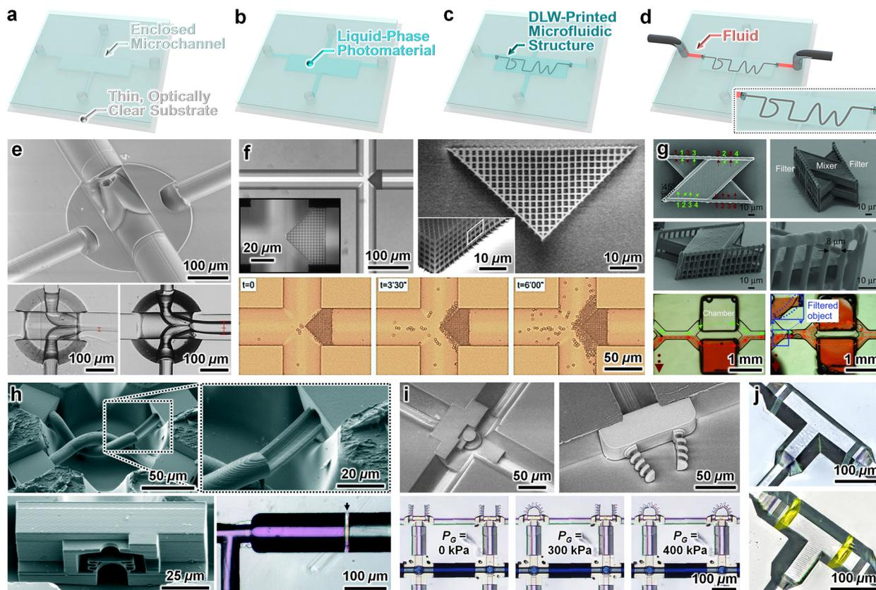
**Fig. 5** Microfluidic systems fabricated by DLW-printing 3D microstructures directly inside (and fluidically sealed to the entire luminal surfaces) of enclosed microchannels—strategies referred to as “*in situ* DLW (*isDLW*)”.
