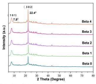
Fig. 4 XRD profiles of all the beta zeolites.
