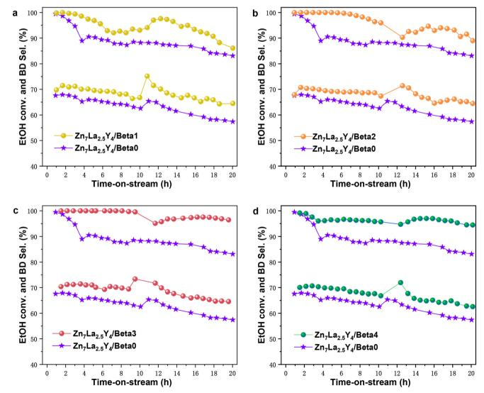
Fig. 6 Ethanol conversion and butadiene selectivity with time-on-stream of (a) Zn<sub>7</sub>La<sub>2.5</sub>Y<sub>4</sub>/Beta1 and Zn<sub>7</sub>La<sub>2.5</sub>Y<sub>4</sub>/Beta0; (b) Zn<sub>7</sub>La<sub>2.5</sub>Y<sub>4</sub>/Beta2 and  $Zn_7La_{2.5}Y_4/Beta0$ ; (c)  $Zn_7La_{2.5}Y_4/Beta3$  and  $Zn_7La_{2.5}Y_4/Beta0$ ; and (d)  $Zn_7La_{2.5}Y_4/Beta4$  and  $Zn_7La_{2.5}Y_4/Beta0$ .
