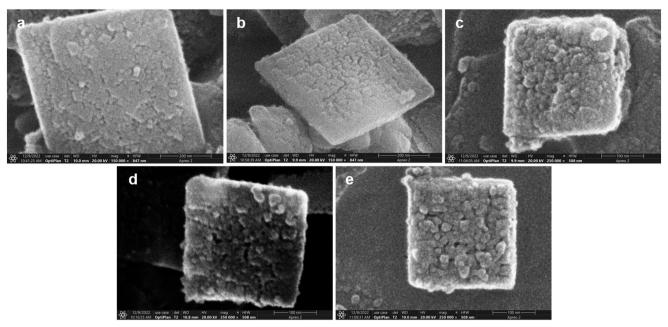
Fig. 1 SEM images of all the beta crystals: (a) Beta0, (b) Beta1, (c) Beta2, (d) Beta3 and (e) Beta4
