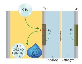
**Fig. 4** Theoretical gas diffusion electrode assembly in flow-by mode for ethylene electrooxidations.
