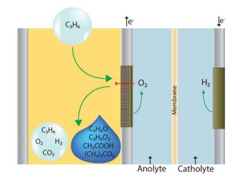
Fig. 11 Theoretical gas diffusion electrode assembly in flow-by mode for propylene electrooxidations.
