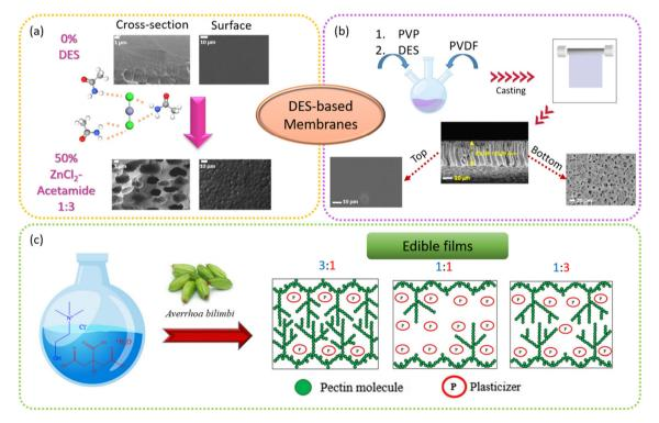
Fig. 10 Illustration of the generation of porous membranes and their SEM images. (a) Polyamide-imide membranes before and after incorporation of ZnCl<sub>2</sub>: acetamide. 164 Copyright 2021, MDPI. (b) With non-ionic DES (N-methyl acetamide: N-methyl urea). 165 Copyright 2022, Elsevier. (c) Schematic illustration of the plasticization effect of edible films generated by Averrhoa bilimbi pectins with a DES. 175 Copyright 2020, Elsevier.
