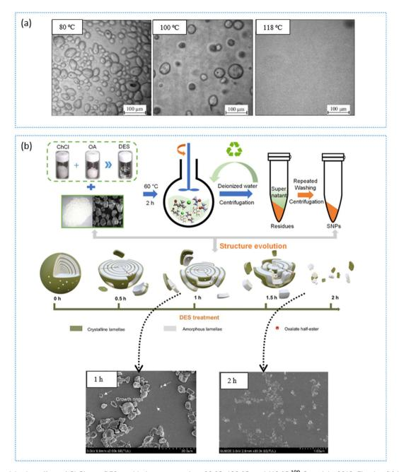
Fig. 5 (a) Plasticization effect of ChCl:urea DES on dried potato starch at 80 °C, 100 °C, and 118 °C. 109 Copyright 2018, Elsevier. (b) Illustration of the formation of starch nanoparticles: DES treatment (ChCl:oxalic acid dihydrate) on waxy maize starch for 1 h and 2 h. 81 Copyright 2022, Elsevier.
