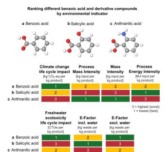
Fig. 3 Comparing the ranking order of three processes producing benzoic acid, salicylic acid and anthranilic acid according to different life cycle impact categories and mass- or energy-based process metrics.
