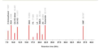
Fig. 7 Separation of various chitin-derived chemicals by HPLC on a Pb<sup>2+</sup> monosaccharide column (analysis conditions: column temperature: 80 °C, mobile phase: water, flow rate: 0.5 mL min<sup>-1</sup>, VWD wavelength: 195 nm).
