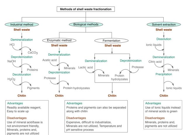
Fig. 4 Methods of shell waste fractionation.
