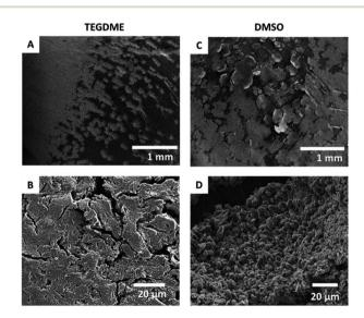
Fig. 8 SEM images of the microstructures formed on applying a 1.0 mA  $cm^{-2}$  constant current in TEGDME (A and B) and DMSO (C and D) at two different magnifications.
