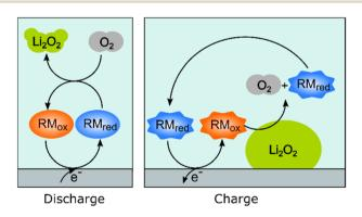
Fig. 3 Schematic representation of how redox-active molecules can be used to aid the discharge and charge processes by enabling oxygen reduction and oxygen evolution reactions (ORR and OER, respectively) to occur chemically in solution as opposed to electrochemically on the surface of the electrode.
