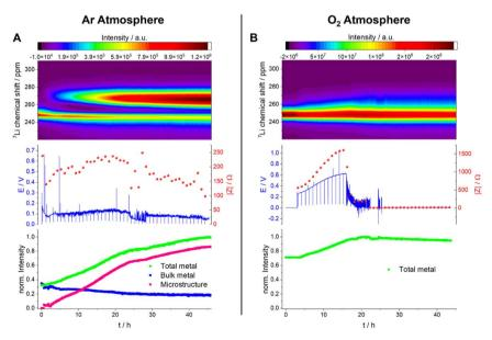
**Fig. 10** Operando NMR spectroscopic measurements of Li-metal plating in symmetrical cells with 1 M LiTFSI in TEGDME under Ar (A) and  $O_2$  (B) atmospheres. Spectra are plotted for the metal signals only in a shift range between 220 and 310 ppm (top) with the corresponding voltage profile and the impedance magnitude |Z| at 9 Hz (middle) and normalised intensity of the metal signal (bottom).
