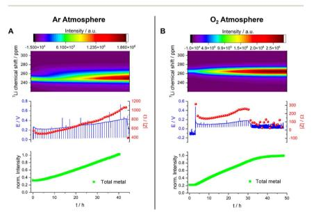
Fig. 11 Operando NMR spectroscopic measurements of Li-metal plating in symmetrical cells with 1 M LiTFSI in DMSO under Ar (A) and  $O_2$  (B) atmospheres. Operando spectra of the metal between 220 and 310 ppm (top) with the corresponding voltage profile and the impedance magnitude |Z| at 9 Hz (middle) and normalised intensity of the metal signal (bottom).
