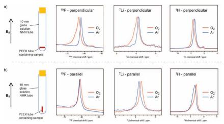
Fig. 1  $^{19}$ F,  $^{7}$ Li, and  $^{1}$ H NMR spectra of a 0.25 M LiTFSI in diglyme electrolyte, where the sample is oriented (a) perpendicular and (b) parallel to the applied magnetic field, before (blue) and after (orange) O<sub>2</sub> saturation, showing the noticeable BMS shifts due to dissolved paramagnetic oxygen. The  $-CH_3$  peak of diglyme is shown for the  $^{1}$ H spectra. Reproduced with permission from ref. 8 under the Creative Commons license CC-BY 4.0, Copyright 2023.
