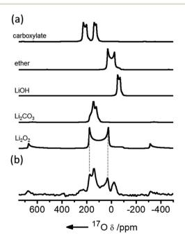
**Fig. 2** (a) Simulated <sup>17</sup>O magic angle spinning (MAS) NMR spectra of possible discharge products compared with (b) the experimental spectrum of a cathode extracted from a cell prepared with a 1 M bis(trifluoromethane)sulfonimide lithium (LiTFSI) electrolyte in dimethoxyethane (DME) solution, after discharge, acquired at a field of 21.1 T and fast (60 kHz) MAS. Reproduced with permission from ref. 9 under the Creative Commons license CC-BY, Copyright 2013.
