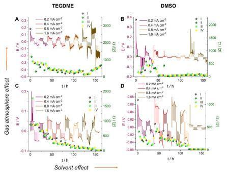
**Fig. 6** The voltage traces of galvanostatic cycling for 1 M LiTFSI electrolyte in TEGDME (A and C) and DMSO (B and D), in Ar (A and B) and  $O_2$  (C and D) atmospheres with currents of 0.2, 0.4, 0.8 and 1.6 mA cm<sup>-2</sup>. The I–IV labels represent different stages in the cycle: (I) nucleation, (II) surface area growth, (III) current direction switch, and (IV) plating on the opposite electrode while stripping the dendrites and stripping bulk lithium, respectively.
