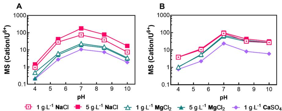
Fig. 5 Membrane selectivity for A) NF90 and B) NF270 based on the transmission ratio of cations to uranium. All solutions in these tests contained  $150 \mu\text{g L}^{-1}$  of uranium (added as  $\text{UO}_2(\text{NO}_3)_2 \cdot 6\text{H}_2\text{O}$ ) and were conducted at  $22^\circ\text{C}$ . pH adjustments were made using 2%  $\text{HNO}_3$  and 1 mM  $\text{NaOH}$ .
