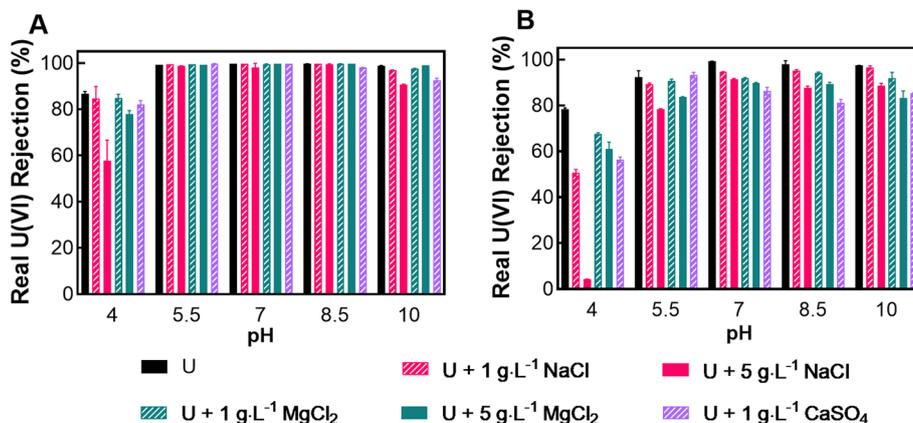
Fig. 3 Comparative uranium rejection by A) NF90 and B) NF270 membranes at different pH levels and ionic conditions. All solutions in these tests contained  $150 \mu\text{g L}^{-1}$  of uranium (added as  $\text{UO}_2(\text{NO}_3)_2 \cdot 6\text{H}_2\text{O}$ ) and operated at  $22^\circ\text{C}$  and 75 psi. Error bars are included to describe the standard error of the mean.
