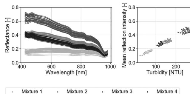
**Fig. 4** Left: overview of the 144 raw wastewater reflectance spectra extracted from the hyperspectral data-cubes (after step 1.4, see Fig. 3). Right: linear relationship between turbidity and mean reflectance intensity.
