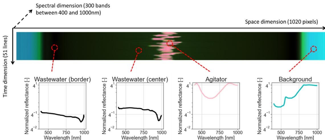
**Fig. 1** Top: typical data-cubes (normalized) with pseudo-RGB colouring corresponding to 380 nm, 500 nm, and 900 nm. One line consists of 1020 pixels, which have a spatial resolution of about 0.1 mm. The image consists of 51 lines collected in 10 seconds. Each image's pixel contains a spectrum ranging from 400 to 1000 nm. Bottom: the spectral dimension is visualized to show the differences between various image areas.
