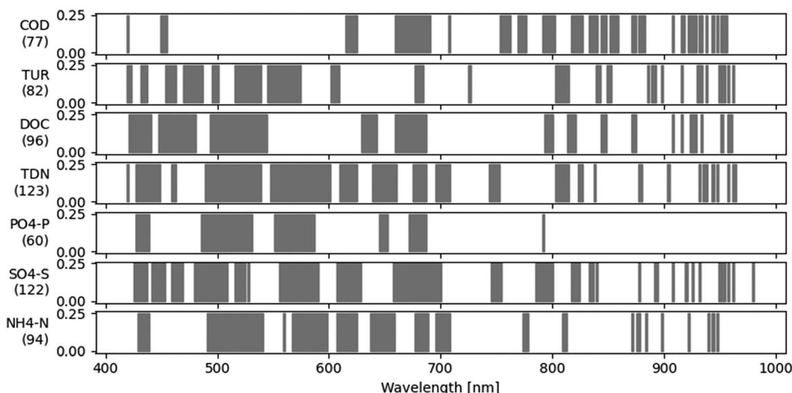
**Fig. 6** Number of selected wavelengths (left, in brackets), PLS weights (dots), and selected wavelengths (grey vertical lines) for each pollution variable. Some patterns are recognizable, but their interpretability is limited (see 3.6).
