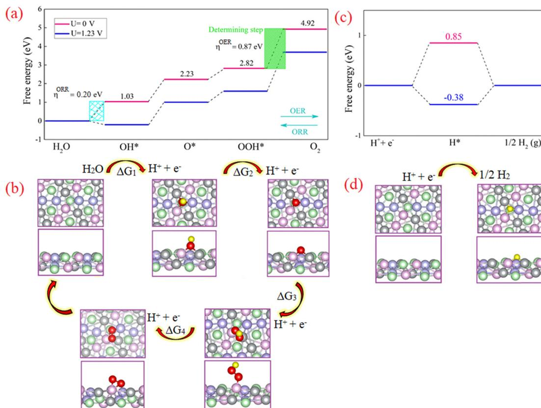
Fig. 6 DFT Studies of the NCMP catalyst. (a) and (c) The calculated free energy diagrams along with (b) and (d) the optimized structure and the microkinetic modeling of the electrocatalytic reaction processes for the (a) and (b) OER, and (c) and (d) HER on the surface of the NCMP catalyst. Color code: Mn (pink), Co (violet), Ni (gray), P (green), O (red), H (yellow).
