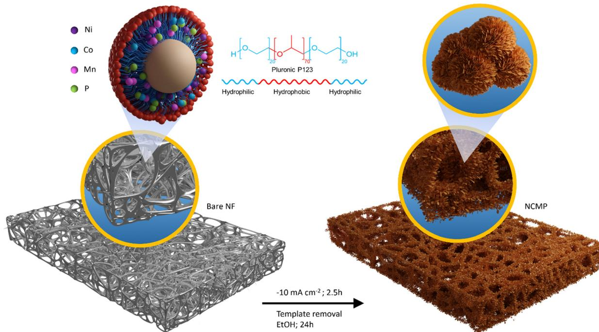
**Fig. 1** Schematic representation of the fabrication process for the NCMP electrode. Schematic illustration of the one-pot and constant current ( $-10 \text{ mA cm}^{-2}$ , 2.5 h) electro-synthesis of the NCMP film on a nickel foam substrate. The chemical structure, amphiphilic character, and the possible morphological transition of Pluronic P123 in aqueous electrolyte, which results in a morphology-controlled electrocatalyst film, is also presented.
