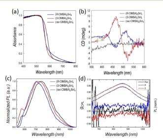
Fig. 24 (a) Absorbance; (b) CD, and (c)  $\mu$ PL spectra of (*R/S/Rac-*CIMBA)<sub>2</sub>SnI<sub>4</sub>. (d)  $g_{CPL}$  (left axis) and static PL (right axis) for (*R/S/Rac-*CIMBA)<sub>2</sub>SnI<sub>4</sub> measured at 90 K. Reprinted with permission from ref. 43 Copyright©2024 Wiley-VCH GmbH.
