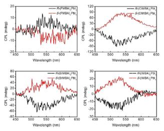
Fig. 7 CPL spectra of (R/S-4-X-MBA)<sub>2</sub>Pbl<sub>4</sub>, X = F, Cl, Br, I. Reprinted with permission from ref. 26 Copyright©2021 Wiley-VCH GmbH.
