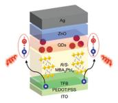
Fig. 38 Pictorical representation of the CISS charge injection for CP-EL emission in the spin-LED device. Reprinted with permission from ref. 66 Copyright © 2023 Wiley-VCH GmbH.
