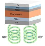
Fig. 33 Schematic representation of the photodiode structure. Reprinted with permission from ref. 57 Copyright © 2023 American Chemical Society.
