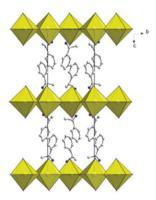
Fig. 3 Packing diagram of (R-MBA)<sub>2</sub>Pbl<sub>4</sub>. Reprinted with permission from ref. 10 Copyright © 2006 Royal Society of Chemistry
