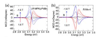
Fig. 17 CD spectra acquired varying the magnetic field from -1.6 to 1.6 T on (a) undoped (R/S-MPA)<sub>2</sub>PbBr<sub>4</sub> and (b) 19% Mn<sup>2+</sup> doped (R/S-MPA)<sub>2</sub>PbBr<sub>4</sub>. Reprinted with permission from ref. 38 Copyright©2024 American Chemical Society
