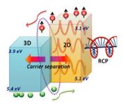
Fig. 35 Pictorial representation of the band alignment of the HOIP heterostructure along with the photogenerated carrier mobility. Reprinted with permission from ref. 60 Copyright © 2021 American Chemical Society.
