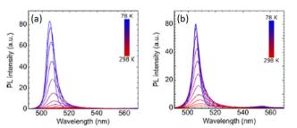
Fig. 11 PL spectra acquired as a function of the temperature for (a) (R-MBA)<sub>2</sub>PbI<sub>4</sub> and (b) (R-pOMeMBA)<sub>2</sub>PbI<sub>4</sub>. Reprinted with permission from ref. 32 Copyright © 2024 American Chemical Society
