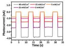
Fig. 32 Photocurrent densities at various incident light intensities of the MAPbl<sub>3</sub>/(R-4-Br-MBA)<sub>2</sub>Pbl<sub>4</sub> device at 785 nm under zero bias. Reprinted with permission from ref. 55 Copyright © 2021 American Chemical Society.
