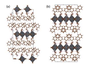
Fig. 19 Crystal structure portion, viewed along the [100] crystallographic direction, of (a) (S-NEA)<sub>2</sub>PbBr<sub>4</sub> and (b) (Rac-NEA)<sub>2</sub>PbBr<sub>4</sub>. Reprinted with permission from ref. 39 Copyright © 2023 Nature Publishing Group
