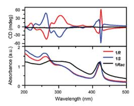
Fig. 21 CD spectra of (R/S/Rac-3AMP)PbBr<sub>4</sub> (above) along with their absorption spectra (below). Reprinted with permission from ref. 41 Copyright@2022 Wiley-VCH GmbH.
