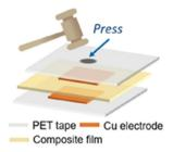
Fig. 37 Schematic representation of the energy harvesting device architecture. Reprinted with permission from ref. 64 Copyright © 2023 American Chemical Society
