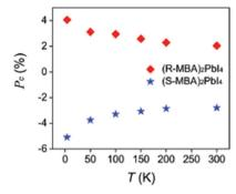
Fig. 8 Temperature-dependent CPL for (R/S-MBA)<sub>2</sub>Pbl<sub>4</sub>. Reprinted with permission from ref. 27 Copyright©2022 Royal Society of Chemistry.
