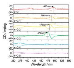
Fig. 6 CD spectra of  $(R/S-MBA)_2Pbl_{4(1-x)}Br_{4x}$ . Solid line, S enantiomer; dashed line, R enantiomer. Reprinted with permission from ref. 23 Copyright@2020 American Chemical Society.
