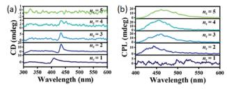
Fig. 28 (a) CD and (b) CPL spectra of (S/R-MBA) $_2$ MA $_{n-1}$ Pb $_n$ Br $_{3n+1}$  as a function of  $\langle n \rangle$ . Reprinted with permission from ref. 48 Copyright ©2022 Wiley-VCH GmbH.
