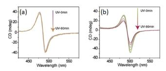
Fig. 10 CD spectra of (a) polymerized and (b) unpolymerized (S-R-MBA)<sub>2</sub>Pbl<sub>4</sub> Reprinted with permission from ref. 30 Copyright © 2023 Wiley-VCH GmbH
