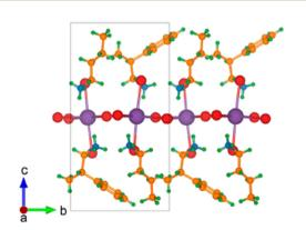
Fig. 16 Crystal structure of (S-MPA)(C<sub>4</sub>A)PbBr<sub>4</sub>, featuring the alternance of S-MPA and C<sub>4</sub>A cations. Reprinted with permission from ref. 37 Copyright@2021 American Chemical Society
