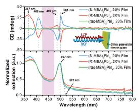
Fig. 4 Transmission CD spectra (above) and normalized extinction spectra (below) of (R/S/Rac-MBA)<sub>2</sub>PbI<sub>4</sub> (in the inset a pictorial representation of a HOIP thin film irradiated by LCP/RCP light). Reprinted with permission from ref. 11 Copyright@2017 Royal Society of Chemistry.
