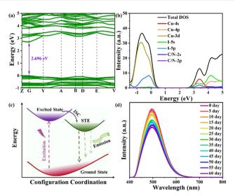
Fig. 3 Electronic band structures (a) and densities of state (b) for the [APCHA]Cu2l4 computed by DFT. (c) Schematic PL mechanism of [APCHA]Cu<sub>2</sub>I<sub>4</sub>. (d) Time-dependent PL spectra of [APCHA]Cu<sub>2</sub>I<sub>4</sub>.
