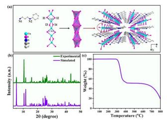
Fig. 1 (a) The detailed and arrangement structure of [APCHA]Cu<sub>2</sub>I<sub>4</sub>. (b) The simulated and experimental PXRD patterns of [APCHA]Cu<sub>2</sub>I<sub>4</sub>. (c) TGA curve of [APCHA]Cu2l4.
