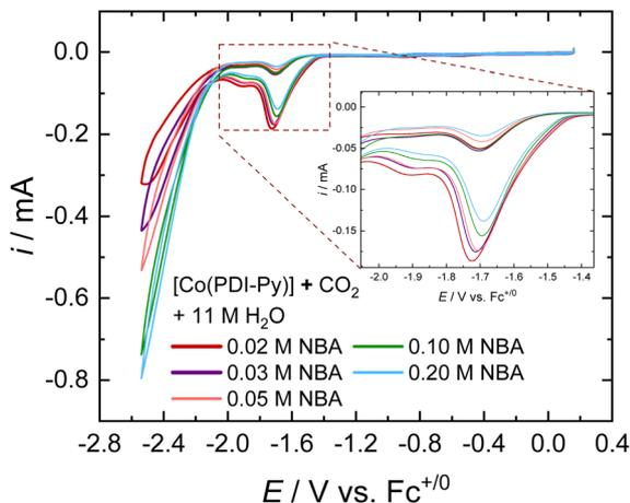
Fig. 2 Representative CVs of 0.3 mM Co(PDI-Py) in MeCN with 0.1 M  $n\text{Bu}_4\text{NPF}_6$  and 11 M  $\text{H}_2\text{O}$  at scan rate of  $0.05 \text{ V s}^{-1}$  with varying concentrations of NBA. The inset is the zoomed in region in the dashed orange box showing the  $e\text{-CO}_2\text{RR}$  catalytic response.
