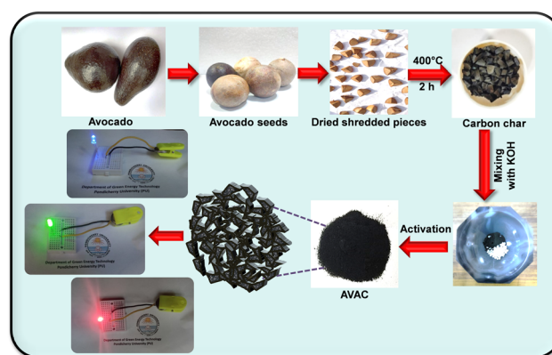
Scheme 1 Schematics of the various steps involved in the generation of the activated carbon from the avocado seed biomass.
