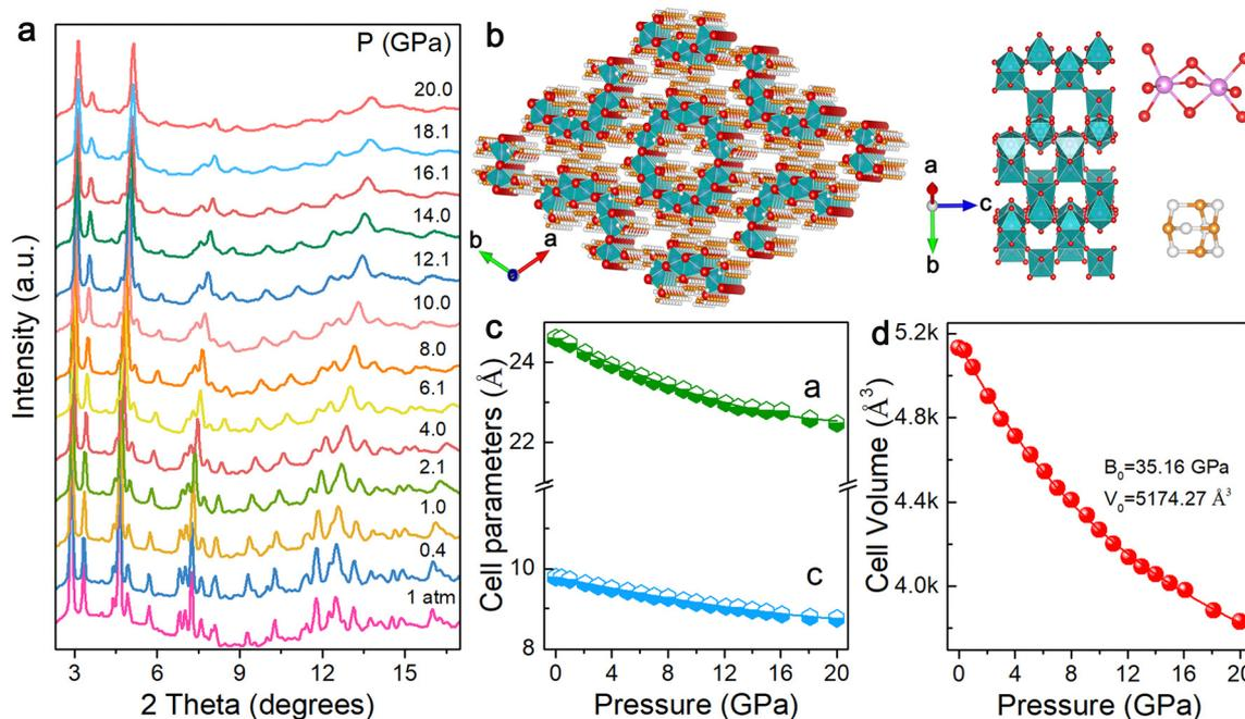
Fig. 3 (a) ADXRD spectra at different pressures. (b) Crystal structure of  $(\text{HMTA})_3\text{Pb}_2\text{Br}_7$ . (Magenta: Pb; red: Br; orange: N; white: C; turquoise polyhedra:  $\text{PbBr}_6$  octahedra and  $\text{Pb}_2\text{Br}_9$  dimers; H atoms have been omitted.) (c) The changes in cell parameters upon compression. (d) Pressure-dependent evolution of unit-cell volumes.
