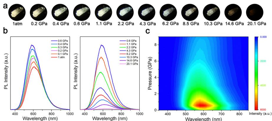
Fig. 1 (a) High-pressure optical PL micrographs of the  $(\text{HMTA})_3\text{Pb}_2\text{Br}_7$  crystal. (b) PL spectra of the  $(\text{HMTA})_3\text{Pb}_2\text{Br}_7$  crystal measured under different pressures. (c) Two-dimensional projection of the PL spectra under high pressure.
