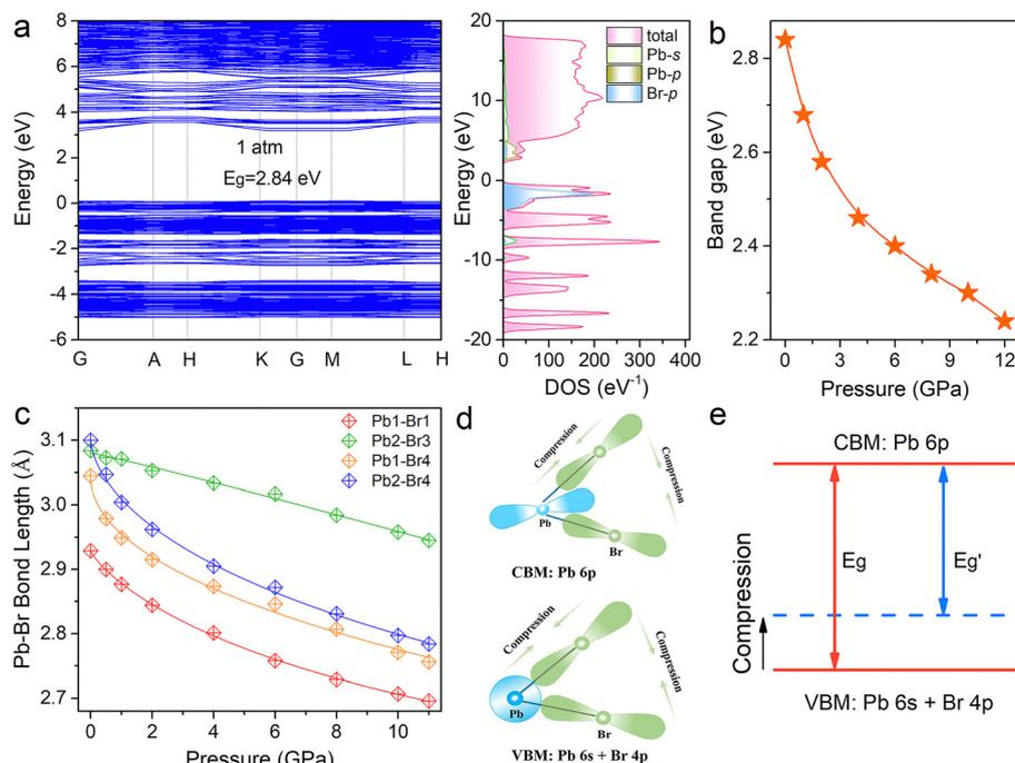
Fig. 4 (a) DFT calculated band structures and projected density of states (DOS) of (HMTA)<sub>3</sub>Pb<sub>2</sub>Br<sub>7</sub> under ambient conditions. (b) Calculated band gap evolution of (HMTA)<sub>3</sub>Pb<sub>2</sub>Br<sub>7</sub> under high pressure. (c) Calculated Pb–Br bond length evolution as a function of pressure. (d) Models of band gap narrowing upon compression. (e) Diagram of the VBM and CBM evolution upon compression.
