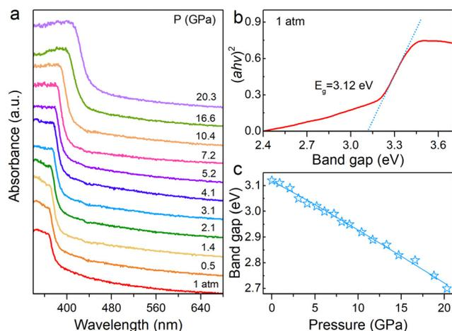
Fig. 2 (a) Evolution of the UV-Vis absorption spectra of the  $(\text{HMTA})_3\text{Pb}_2\text{Br}_7$  crystal at selected pressures. (b) The Tauc plot of  $(\text{HMTA})_3\text{Pb}_2\text{Br}_7$  under ambient conditions. (c) Demonstration of the band-gap narrowing in  $(\text{HMTA})_3\text{Pb}_2\text{Br}_7$  at high pressures.
