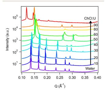
Fig. 5 SAXS patterns of 10 wt% phytantriol in mixtures of water and ChCl:U at 25  $^{\circ}$ C. Data for the solvent mixture of 70/30 ChCl:U/water has been omitted for clarity. Data are offset vertically for clarity.
