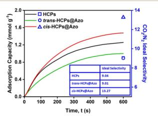
Fig. 3 CO<sub>2</sub> adsorption profiles of (black) HCPs, (green) visible light irradiated *trans*-HCPs@Azo and (red) UV light irradiated *cis*-HCPs@Azo using a flow rate of 10 mL min $^{-1}$ , pure CO<sub>2</sub> gas, at room temperature and atmosphere pressure. CO<sub>2</sub>/N<sub>2</sub> ideal selectivities of HCPs, *trans*-HCPs@Azo and *cis*-HCPs@Azo were obtained using CO<sub>2</sub> and N<sub>2</sub> pure gas adsorption capacities after 600 s (Table S2†). <sup>43,44</sup>
