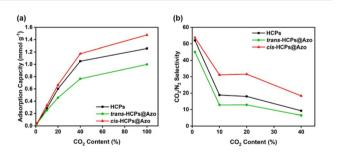
Fig. 4 (a)  $CO_2$  adsorption capacities and (b) mixed gas  $CO_2/N_2$  selectivities (Table S3†)<sup>51,52</sup> of (black) HCPs, (green) *trans*-HCPs@Azo and (red) *cis*-HCPs@Azo at different  $CO_2$  concentration of 1 v/v%, 10 v/v%, 20 v/v%, 40 v/v% and 100 v/v% at room temperature (25 °C) and atmosphere pressure (1 bar).
