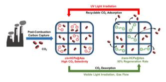
Fig. 1 Our approach of exploiting photo-isomerisation of azobenzene molecules embedded in pores of HCPs to drive adsorption (upon UV irradiation) and desorption (vis-irradiation) of  $CO_2$  to enable low-energy, low-cost carbon capture.
