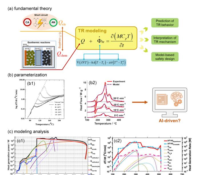
Fig. 4 Thermal runaway modelling of lithium(-ion) batteries. (a) Fundamental theory for battery TR modelling. (b) Parameterization of the exothermic reactions based on the (b1) ARC and (b2) DSC test data. Reproduced with permission from ref. 39 and 40. Copyright 1999, IOP Publishing, and Copyright 2018, Elsevier. (c) Model-based analysis of the battery TR mechanism. Modified with permission from ref. 41 (c1) and 42 (c2). Copyright 2018, IOP Publishing, and Copyright 2022, Elsevier.
