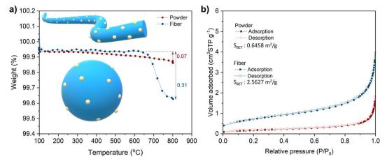
Fig. 4 Exsolution process of LCNT perovskite materials under chemical reduction. (a) Weight loss of LCNT samples reduced in  $5\% H_2/N_2$  from 100 to 800 °C, (b) N<sub>2</sub> adsorption-desorption isotherms and BET surface area of samples.
