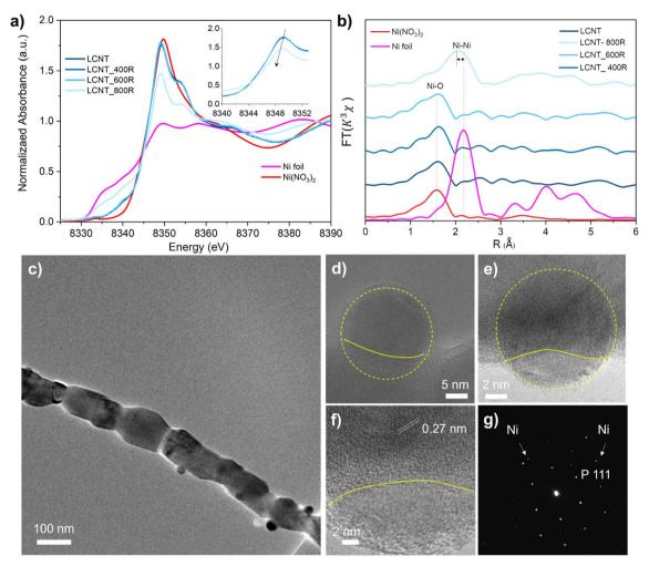
Fig. 3 Characterization and microstructure of reduced LCNT perovskite fibers. (a) Ni K-edge XANES spectra and (b) Fourier-transformed  $k^3x$  data for fibers reduced at 400, 600, and 800 °C with standard samples of Ni foil and Ni(NO<sub>3</sub>)<sub>2</sub>. (c) TEM images of reduced fiber. (d–f) TEM image of exsolved particle, (g) the corresponding SAED pattern of (c).
