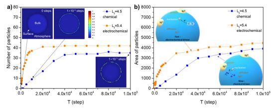
Fig. 6 Phase-field simulation results for exsolution. (a) The number of particles and the exsolution particles profile vs. steps from the model, the insets show the contour plots of exsolved particles. (b) The area of particles and schematic of bias-driven exsolution of nanoparticles from perovskite fiber cells, the insets corresponding to the exsolution process under electrochemical and chemical driven, respectively.
