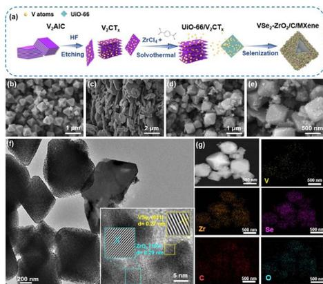
Fig. 1 (a) Schematic of the preparation of  $VSe_2-ZrO_2/C/MXene$ . FESEM images of (b)  $Se-ZrO_2/C$ , (c)  $VSe_2/MXene$  and (d) and (e)  $VSe_2-ZrO_2/C/MXene$ . (f) TEM (inset: HRTEM and corresponding IFFT image), and (g) EDS elemental mapping images of  $VSe_2-ZrO_2/C/MXene$ .
