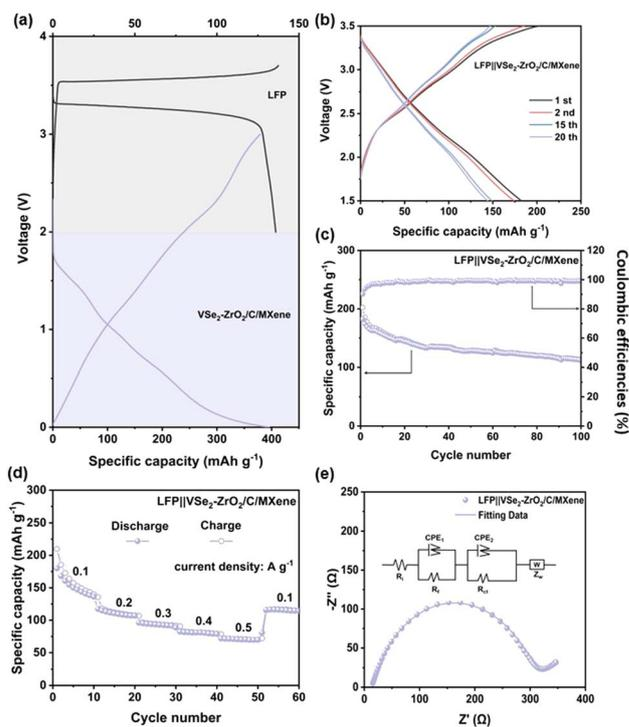
Fig. 8 (a) Half-cell charge–discharge profiles of LFP and  $\text{VSe}_2\text{-ZrO}_2/\text{C}/\text{MXene}$  electrodes at  $100 \text{ mA g}^{-1}$ . (b) Galvanostatic charge/discharge profiles and (c) cycling performances for  $\text{LFP}\|\text{VSe}_2\text{-ZrO}_2/\text{C}/\text{MXene}$  full cell at  $100 \text{ mA g}^{-1}$ . (d) Rate performances and (e) Nyquist plot for  $\text{LFP}\|\text{VSe}_2\text{-ZrO}_2/\text{C}/\text{MXene}$  full cell (inset: equivalent electrical circuit model).
