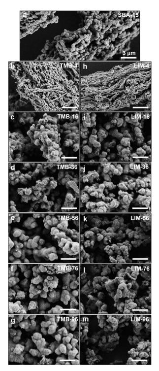
Fig. 5 SEM images of SBA-15 (a) and pore expanded micellar templated silica obtained with increasing amounts of expander TMB (left column) and limonene (right column). The scale bar is 3 µm for all images.
