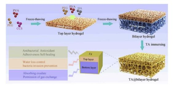
Fig. 7 Preparation process of TA@bilayer hydrogel.85
