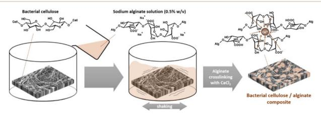
Fig. 8 Fabrication of bacterial cellulose/alginate composite. 130
