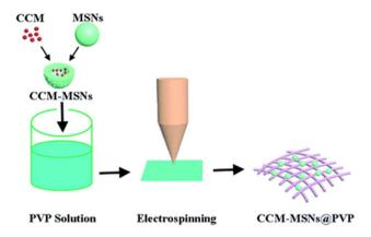
Fig. 4 Fabrication of curcumin-loaded mesoporous silica nanofiber mats.114
