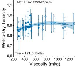
Fig. 10 Strength properties of the spun fiber as a function of pulp viscosity. Left: conditioned tenacity, right: ratio between conditioned and wet tenacities (closed circles: HWPHK pulps; open circles: SWS-IP pulps).
