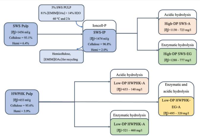
Scheme 1 Schematic flow diagram of the pretreatment of SWS and HWPHK pulps for the production of dissolving pulps with a broad DP spectrum and different molecular weight distributions (MWDs).
