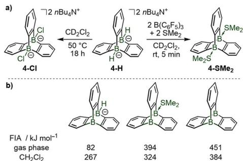
**Scheme 3** Reactivity of the 9,10-diboratriptycene dihydride **4-H**: activation of the B–H bonds and coordination of the bridgehead boron atoms with anions or Lewis bases via the generation of transient pyramidal boron Lewis acids. Fluoride ion affinities computed at the PBE0-D3(BJ)/def2-TZVPPD theory level using isodesmic reactions with COF<sub>2</sub> anchor point, values from ref. 4.
