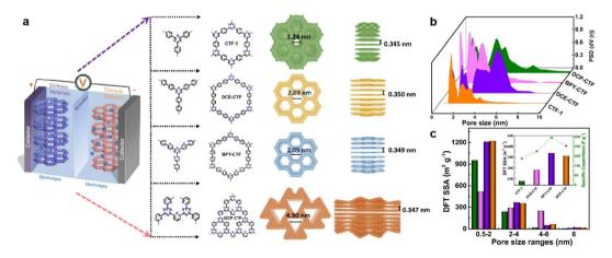
Fig. 10 (a) Schematic diagram of supercapacitor configuration together with design and synthesis of CTF-1, DCE-CTF, BPY-CTF and DCP-CTF, including the top and side views from left to right. (b) The pore size distribution calculated by QS-DFT for CTF-1, DCE-CTF, BPY-CTF, and DCP-CTF. (c) DFT SSA distribution of different pore size ranges, the inset is DFT SSA of CTFs derived from pores with size range of 2–4 nm *versus* specific capacitance. Reprinted from ref. 95. Copyright 2022, Elsevier.
