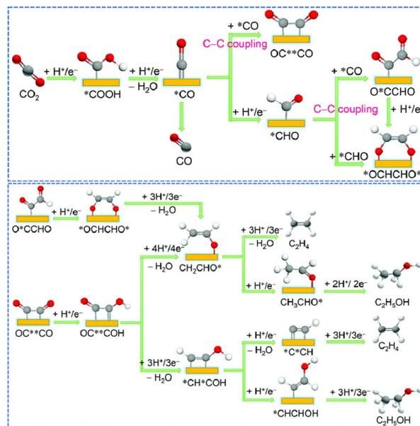
Fig. 3 Possible C–C coupling mechanisms in the electrocatalytic  $\text{CO}_2$  reduction (above). Mechanisms of forming  $\text{C}_2\text{H}_4$  and  $\text{C}_2\text{H}_5\text{OH}$  after C–C coupling (below). Reproduced from ref. 92. Copyright 2021 Royal Society of Chemistry.
