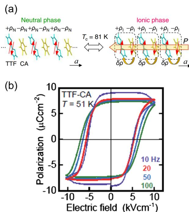
Fig. 9 (a) Schematic illustration of the neutral-to-ionic transition in TTF-CA (TTF = tetrathiafulvalene, CA = *p*-chloranil).  $P$  is the ferroelectric polarization.<sup>57</sup> Reproduced from ref. 57. (b) Hysteresis loops of TTF-CA with various frequencies at 51 K.<sup>50,52</sup> Reproduced with permission from ref. 50, American Physical Society.
