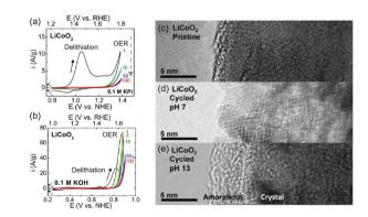
Fig. 4 Cyclic voltammogram (CV) of LiCoO<sub>2</sub> (LCO) in (a) neutral and (b) alkaline electrolytes. (c-e) TEM image of LCO (c) pristine, (d) after cycling at pH 7, and (e) after cycling at pH 13. Adapted with permission from ref. 89. Copyright 2012 American Chemical Society.
