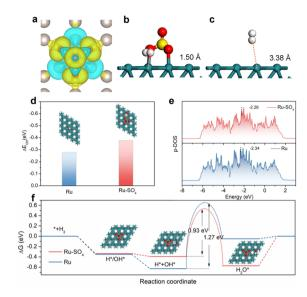
Fig. 4 (a) Calculated differential charge density for  $Ru-SO_4$ . The blue and yellow areas correspond to the depletion and accumulation of electrons, respectively. The optimal theoretical structure of  $H_2$  on  $Ru-SO_4$  (b) and Ru (c). (d) The adsorption energy of  $OH^*$  on  $Ru-SO_4$  and Ru with the corresponding optimal theoretical structure. The projected density of states (e) and the reaction pathways (f) of Ru and  $Ru-SO_4$ .
