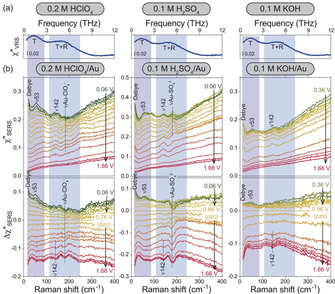
Fig. 2 (a)  $\chi''_{\text{VRS}}$  spectra for bulk aqueous solutions containing different electrolytes. (b) Potential dependence of  $\chi''_{\text{SERS}}$  spectra for the respective electrolyte solutions on Au surfaces (upper panel) and their  $\Delta\chi''_{\text{SERS}}$  spectra with respect to pzc for each solution (bottom).
