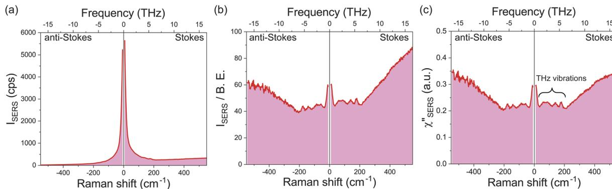
Fig. 1 A raw SERS spectrum for the 0.1 M  $\text{H}_2\text{SO}_4/\text{Au}$  interface covering both Stokes and anti-Stokes branches, measured on an electrochemically roughened Au surface using 632.8 nm excitation. (b) Reduction of the Bose–Einstein thermal factor and frequency factor in (a). (c) Reduction of the Purcell factor in (b), which corresponds to the  $\chi''_{\text{SERS}}$  spectrum composed of the vibrational and electronic responses at the interface in a density of states format.
