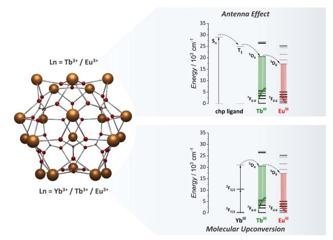
Fig. 7 Metal core structure of the  $\{Ln_{20}\}$  MCAs (CCDC number: 2023766)<sup>81</sup> and the energy transfer mechanism for antenna effect and UC emissions. <sup>81,95</sup> Colour code: Dark orange: Ln<sup>3+</sup>; grey: carbon; red: oxygen. Hydrogen atoms were omitted in the structure for clarity.
