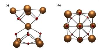
Fig. 4 Metal core structure for {Ln<sub>9</sub>} MCAs. (a) Side view and (b) top view. CCDC number: 956639.<sup>80</sup> Colour code: Dark orange: Ln<sup>3+</sup>; red: oxygen. Hydrogen atoms were omitted in the structure for clarity.
