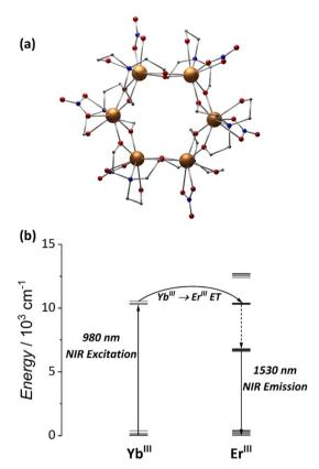
Fig. 5 (a) Single-crystal structure for {Ln<sub>6</sub>} MCAs (CCDC number: 1958091). (b) Energy-transfer mechanism for the NIR-to-NIR emission.<sup>79</sup> Colour code: Dark orange: Ln<sup>3+</sup>; grey: carbon; red: oxygen; blue: nitrogen. Hydrogen atoms were omitted in the structure for
