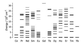
Fig. 2 Partial energy-levels diagram for trivalent lanthanides. Energies obtained from Carnall.<sup>99</sup>
