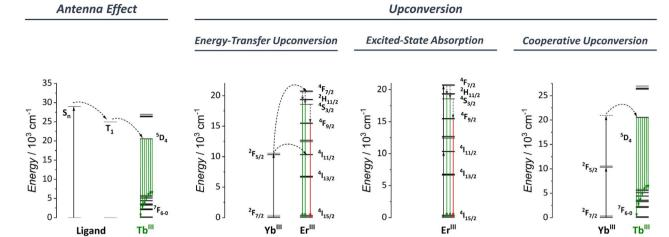
Fig. 3 Depiction of some commonly observed luminescence mechanisms for  $Ln^{3+}$  ions. From left to right: Ligand-based antenna effect,  $Yb^{3+}$ - $Er^{3+}$ -based energy-transfer upconversion,  $Er^{3+}$ -based excited-state absorption, and  $Yb^{3+}$ - $Tb^{3+}$ -based cooperative upconversion.
