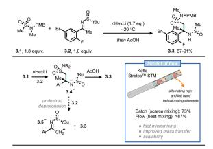
Fig. 3 Adoption of flow chemistry in an industrial setting allows to avoid undesired fast deprotonation in the synthesis of **3.3**, an intermediate for the manufacturing of verubecestat (MK-8931). STM: static tube mixer.
