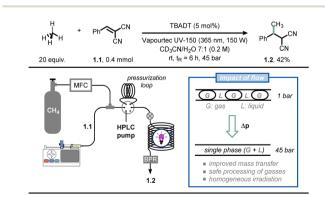
Fig. 1 Microflow technology improves gas—liquid mass transfer, which can be exploited for the functionalization of gaseous light hydrocarbons. TBADT: tetrabutylammonium decatungstate; BPR: back-pressure regulator; MFC: mass-flow controller.
