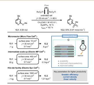
Fig. 13 Adoption of flow electrochemistry in an industrial context for the highly scalable, selective anodic oxidation of thioether 13.1.  $t_{recirc}$ : time of recirculation.
