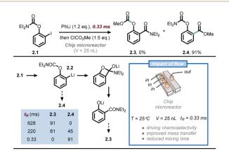
Fig. 2 Ultra-fast mixing provided by flow technology allows to outpace undesired anionic Fries rearrangement in the functionalization of iodophenyl carbamates at the *ortho* position. t<sub>R</sub>: residence time.
