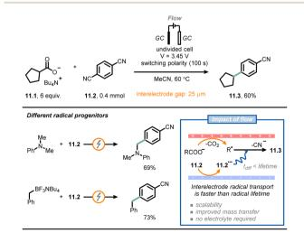
Fig. 11 Microfluidic electrochemical cells with short inter-electrode gaps enable redox-neutral transformations in the absence of supporting electrolytes. GC: glassy carbon.
