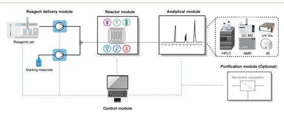
Fig. 20 General configuration of an automated and modular continuous-flow platform.
