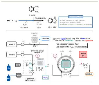
Fig. 15 Continuous-flow setup for the generation of  $N_2O_3$  and its subsequent use in synthetically-relevant contexts. CV: check valve; 6PV: six-position switch valve. MFC: Mass-Flow Controller. Reproduced from ref. 83 with the permission of Wiley-VCH, copyright 2022.
