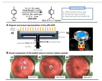
Fig. 19 Scale up of the [4 + 2] cycloaddition between terpinene and photochemically generated singlet oxygen using rotor-stator spinning disk reactor technology. Reproduced from ref. 93 with the permission of Elsevier, copyright 2020.
