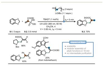
Fig. 9 Use of flow chemistry to devise a flexible approach for the installation of allyl moieties at strong aliphatic  $C(sp^3)$ -H bonds.
