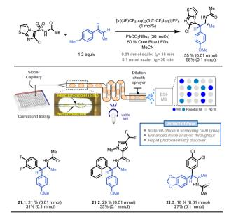
Fig. 21 Development of a droplet-based flow-HTE platform to prepare API libraries in a time- and resource-efficient fashion. Reproduced from ref. 121 with the permission of Springer Nature, copyright 2020.
