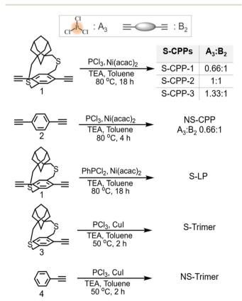
Scheme 1 Synthesis of strapped CPPs (S-CPP-1–3), non-strapped CPP (NS-CPP), strapped linear polymer (S-LP), and model trimers (S-trimer & NS-trimer).
