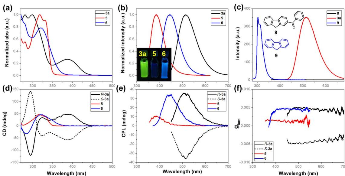
Fig. 2 (a) UV-vis and (b) fluorescence spectra of **3a**, **5**, and **6** in  $\text{CH}_3\text{CN}$ ; (c) fluorescence spectra of **3a** ( $2 \times 10^{-5}$  M), **8** ( $2 \times 10^{-5}$  M), and **9** ( $5 \times 10^{-6}$  M) in  $\text{CH}_3\text{CN}$ ; (d) ECD and (e) CPL spectra of *P*-**3a**, *M*-**3a**, **5**, and **6** in  $\text{CH}_3\text{CN}$  ( $5 \times 10^{-5}$  M); (f) luminescence dissymmetry factors  $g_{lum}$  of *P*-**3a**, *M*-**3a**, **5**, and **6**.
