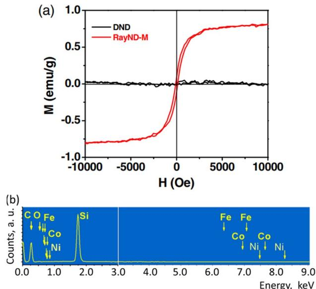
Fig. 10 Magnetic properties of RayND-M ( $d = 4.3\text{--}4.5$  nm). (a) Magnetization curve of RayND-M [in comparison with ordinary detonation ND (DND),  $d = 3\text{--}10$  nm]. (b) EDS spectrum of RayND-M; Fe, Co, and Ni atoms as impurities were not detected.<sup>139</sup> Reproduced with permission from ref. 139 Copyright 2018 SPIE.
