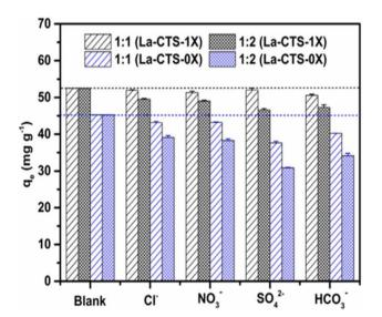
Fig. 4 Effect of coexisting ions on  $PO_4^{3-}$  recovery by La-CTS-1X and La-CTS-0X (the ratios of the initial  $PO_4^{3-}$  concentration to the coexisting ion concentration are 1:1 and 1:2). Reproduced with permission from ref. 96 with permission from Elsevier, copyright 2019.
