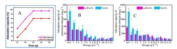
Fig. 10 (A) The effect of PEG/chitosan and PVA/chitosan composite dose on  $NO_3^-$  adsorption<sup>101</sup> with permission from Elsevier, copyright 2016. (B) The effect of Fe–Cs and La/Fe–Cs composite dose on ammonium–nitrogen removal from cow breeding wastewater and (C) pig farm wastewater. Reproduced with permission from ref. 1 with permission from Elsevier, copyright 2022.
