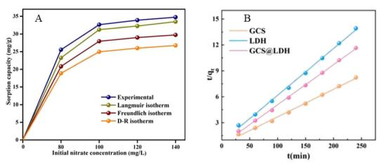
Fig. 11 (A) Experimentally measured isotherms for NO<sub>3</sub><sup>-</sup> adsorption by Zr@AlgKN composite beads. Reproduced with permission from ref. 86 with permission from Elsevier, copyright 2020. (B) Pseudo-second-order model on NO<sub>3</sub><sup>-</sup> removal by GCS, LDH, and GCS@LDH. Reproduced with permission from ref. 104 with permission from Elsevier, copyright 2022.
