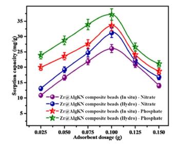
Fig. 5 Effect of adsorbent dose on adsorption capacity of *in situ* and hydrothermal synthesized Zr@AlgKN composite beads towards  $NO_3^-$  and  $PO_4^{3-}$ . Reproduced with permission from ref. 86 with permission from Elsevier, copyright 2020.
