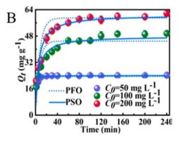
Fig. 6 (A) The Langmuir and Freundlich isotherm models and (B) pseudo-first-order and pseudo-second-order kinetics models for the adsorption of  $PO_4^{3-}$  on La/Fe–Cs composites. Reproduced with permission from ref. 1 with permission from Elsevier, copyright 2022.
