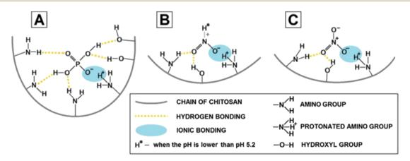
Fig. 7 Possible mechanisms of nutrient bonding onto chitosan sorbents: (A) PO<sub>4</sub><sup>3-</sup>, (B) N-NO<sub>2</sub>, and (C) N-NO<sub>3</sub>. Reproduced with permission from ref. 92 with permission from Elsevier, copyright 2017.
