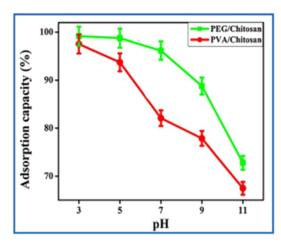
Fig. 8 Effect of pH on adsorption of NO<sub>3</sub><sup>-</sup> by PEG/Cs and PVA/Cs. Reproduced from ref. 101 with permission from Elsevier, copyright
