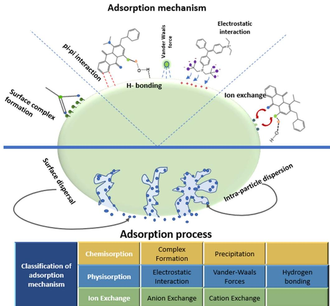
Fig. 6 Brief representation of the classification of adsorption mechanisms adopted by the dye removal process.<sup>223</sup>
