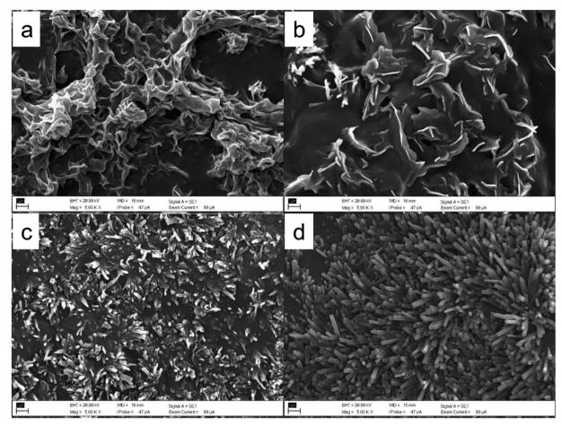
Fig. 2 SEM micrographs of wheat straw wax recrystallized by different solvents, (a) petroleum ether, (b) toluene, (c) TMO, and (d) DEDMO. Scale bars: 1 µm.
