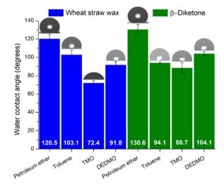
Fig. 6 Water contact angle measurement for wheat straw wax and  $\beta$ -diketone recrystallized by different solvents.
