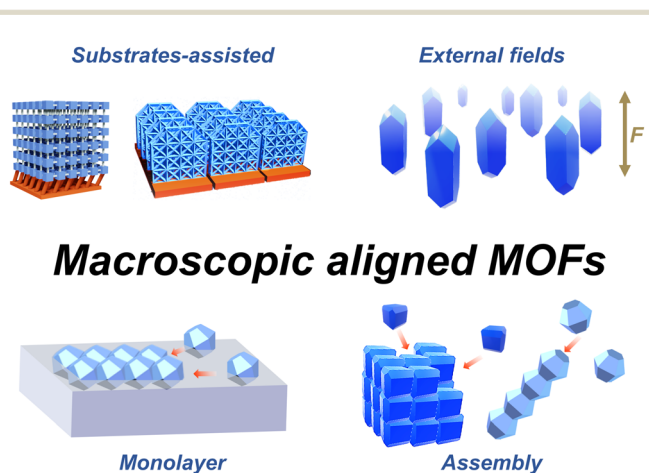
Fig. 1 Schematic illustration of a variety of methods for preparing macroscopic aligned MOFs.
