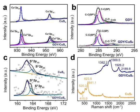
High-resolution (a) Cu 2p, (b) C 1s, and (c) S 2p XPS spectra of CuS<sub>x</sub> and GDY/CuS<sub>x</sub>. (d) Raman spectra of CuS<sub>x</sub> and GDY/CuS<sub>x</sub>.
